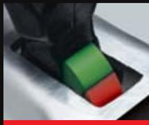
The coloured wear indicator on the coupling handle indicates the condition of the towball. If the red segment is visible, then the towball has worn and should be replaced.
